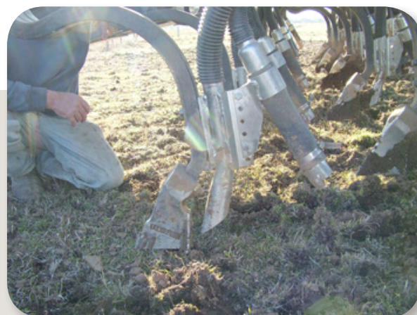
The important parts of the Agrowdrill®. The boot cuts a slot. The deep tube is for fertiliser and the shorter tube at the back sows the seed. This machine does not have presswheels but uses a finger roller to press the seed into the slot and maximise soil-seed contact. Loose rings on the roller allow the fingers on the roller to stay in the rows.
